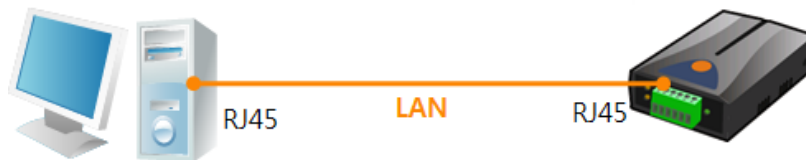
Figure 2-1 the connection between CIE-H12 and a PC
