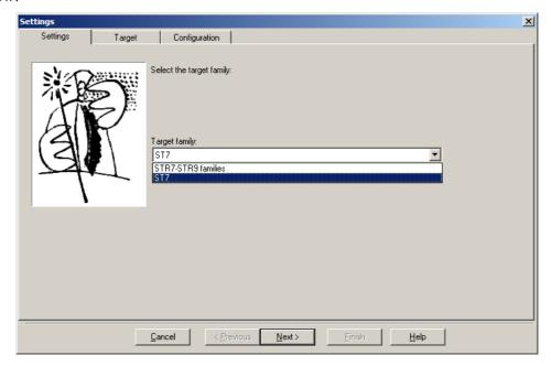
Select your target family, then click "Next" to go to the target tab. In the Target tab, select your target derivative and note the start address for the flash memory shown in the device description, then click "Next".
