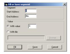
Enter the start and end addresses, then select "with file" and click on "Browse...". Here you can enter a file name such as "dump.hex", and click on "Open". Back in the "Fill or Save segment" dialog box, click on the "Save" button. The file dump.hex is created, containing the memory dump in Intel HEX format.
