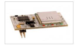
FLYPORT is powered by openPicus framework based on FreeRTOS. The free IDE allows to create applications, to import web pages and to compile and download code to the module.
