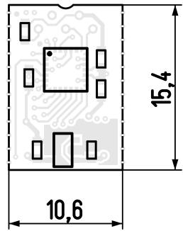
Height at thickest point: max. 2.2 mm
