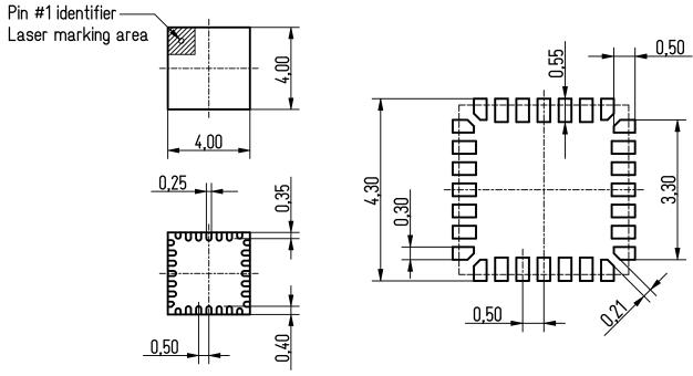
Package thickness: 0.55 mm ±0.05 mm Outer contour tolerance: ±0.1 mm
